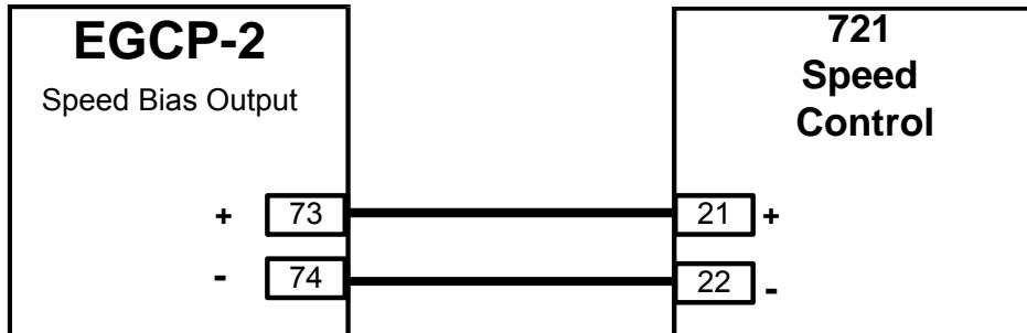
EGCP-2 To 701 and 701A Wiring and Configuration Settings
